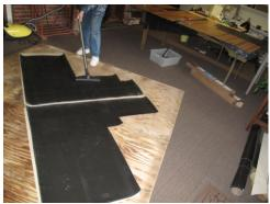
delivered with Amtico, have the strips bonded directly to the plywood sole without additional soundproofing. We thought adding the weight was worth it because reducing engine noise was a secondary goal.
