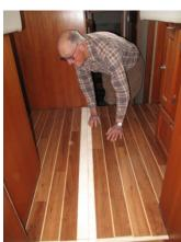
panels to the sole, and nailed the panel to sole everywhere panel's plywood core was still exposed (along central fore-aft joint and various exposed cut-outs).
