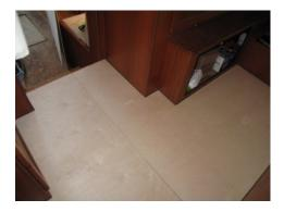
referenced off a clamped fence for every straight cut – made for extremely accurate straight square, splinter free edges (there is <u>a lot</u> of precise handling of these heavy panels later). Using a saber saw would have left a nasty splintered edge.
